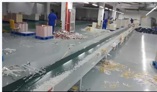
Packaging production line connected to shredding equipment
